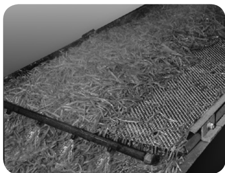
Vibrating screen being used in vegetable processing.
