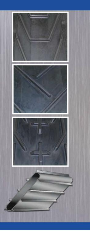
**THE BIGHORN** belt offers a 3/4" high x 3/4" thick rounded at the top cleat on 9" centers. This belt is ideal for smooth delivery of loads requiring a cleated belt for elevation of product up steep inclines. The Bighorn maintains constant contact with return idlers and can be troughed on conventional troughing idlers.
