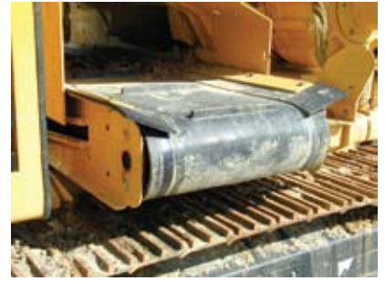
Skirtboard Rubber On Trencher
