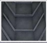
**THE BIGHORN** belt offers a 3/4" high x 3/4" thick rounded at the top cleat on 9" centers. This belt is ideal for smooth delivery of loads requiring a cleated belt for elevation of product up steep inclines. The Bighorn maintains constant contact with return idlers and can be troughed on conventional troughing idlers.
